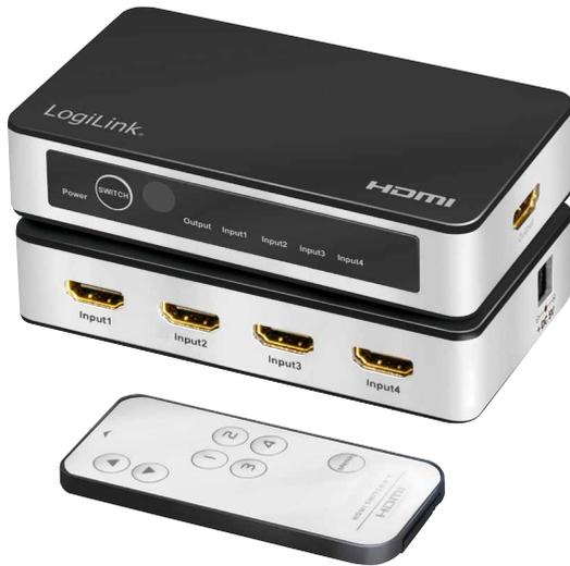
Designed for applications that require the routing of 4 sources to 1 compatible display device. It enables the reliable transmission at video resolutions up to 4K@60 Hz. Features auto and manual switching modes for selection; instantly switching for a smooth video transition between HDMI ports.
