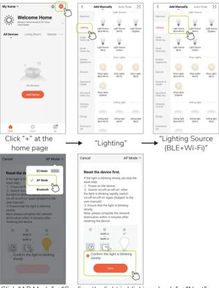
Click "AP Mode"  $\rightarrow$  "Confirm the light is blinking slowly"  $\rightarrow$  "Next". If you see the rapid blinking instead of slow ones, reset to AP mode by turning OFF/ON 3 times.
