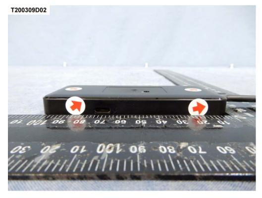
Red Dot —Air Discharged Blue Dot —Contact Discharged
